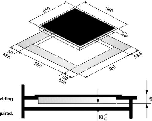
When installing the cooktop above a cupboard, a dividing shelf as pictured above must be installed.
