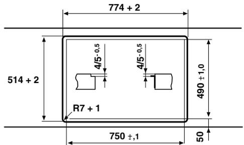
Installation when using supporting angles or strips of wood or stone.
