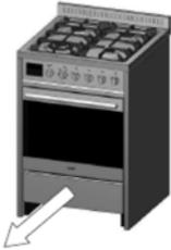
2 - Place the Kick Plate and press the pins directly into the holes:
