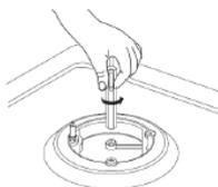
3 - Replace all burner component and the pan supports.
