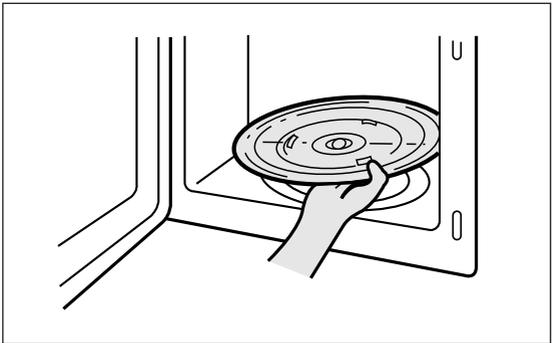
7. The roller guide and oven cavity floor should be cleaned regularly to avoid excessive noise.
